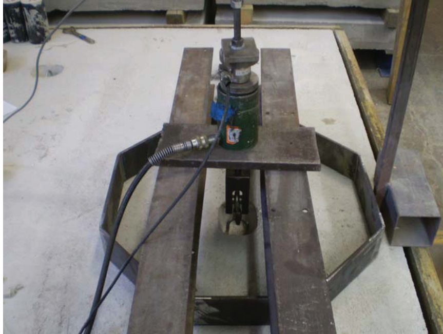
Figure 2 - Pull-Out Test set up
