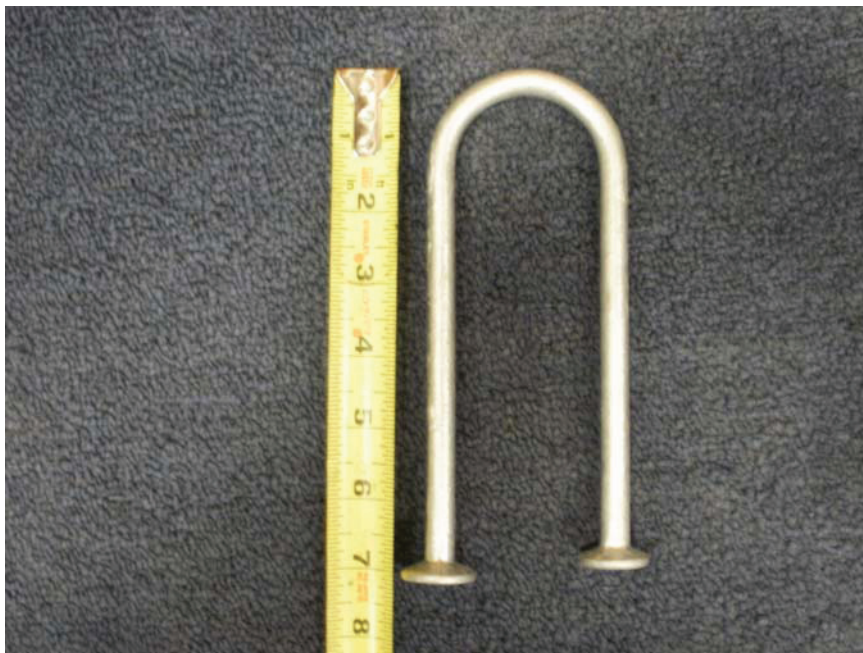
Figure 3 – Anchor component un-cast
